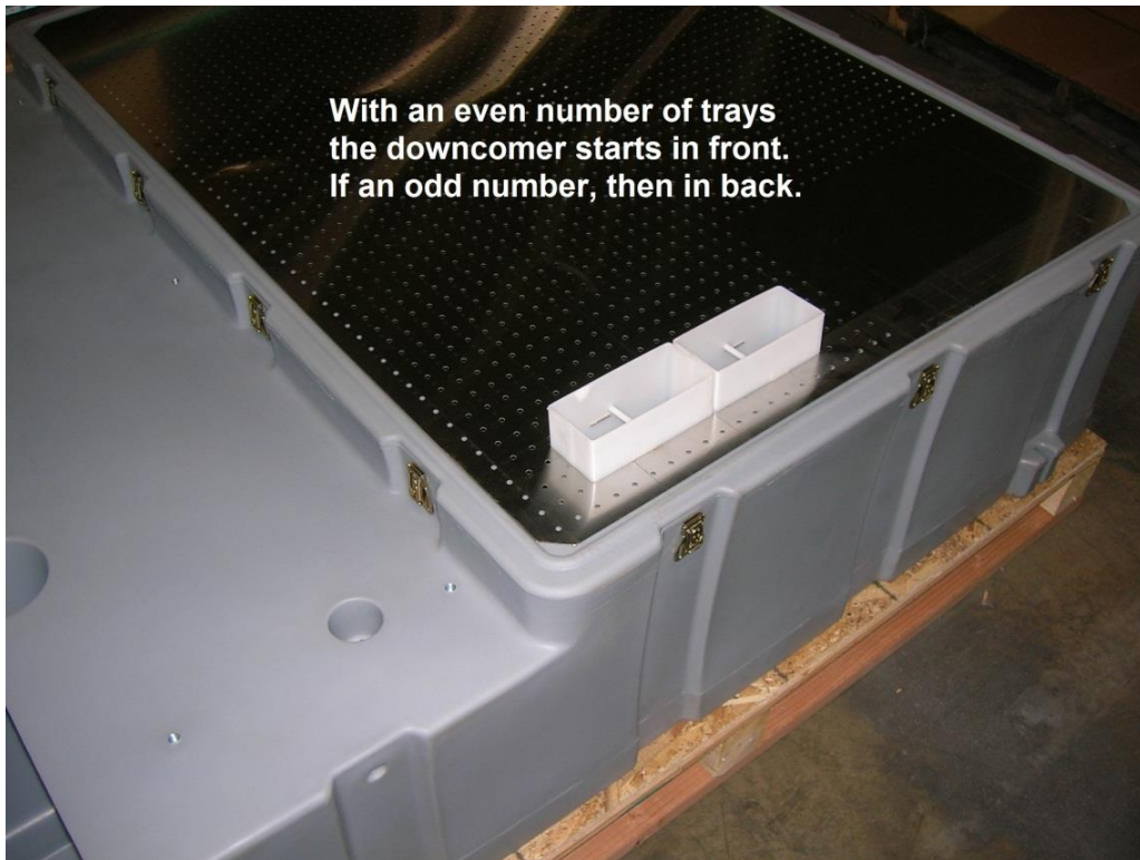
Figure 4-6: First Bubble Plate on LO-PRO III Sump
